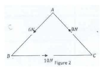
Forces of 10N, 8N and 6N act along the sides BC, CA and AB of an equilateral triangle ABC as in figure 2. Find the magnitude of the resultant of these forces and the angle which it makes with BC.
