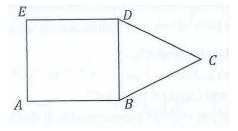
Figure 1 is a uniform density lamina ABCDE, made from a square of side 2a and equilateral triangle of side 2a. Show that the distance of the centriod of lamina from BD is
