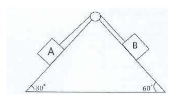
Two particles *A* and *B*, of masses 2*m* and 6m, rest on the smooth and rough inclined faces respectively of a fixed wedge as in Fig. 1. They are connected by a flight inextensible string passing over a smooth pulling fixed at the top of the wedge. The smooth face of the wedge is inclined at angle 30° to the horizontal while the rough face is inclined at angle 60° to the horizontal. The system is released from rest with the string taut. Given that the
