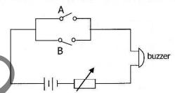
Which gate is represented by the combination of switches A and B?
