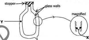
Which processes of heat transfer do parts X and Y affect?
